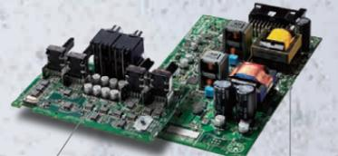
Pre-Amplifier Circuit Power Amplifier Circuit
